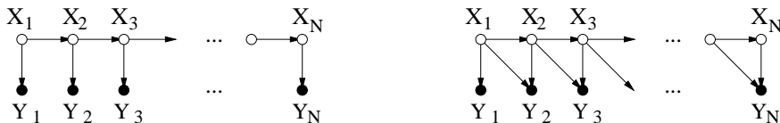
Figure 2: A Markov process X and a measurement process Y , on variables of X (left-hand side) or on transitions of X (right-hand side).
